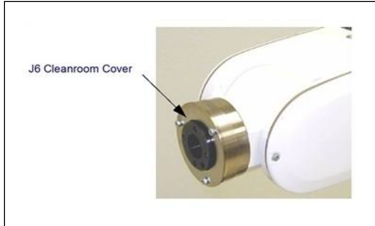
Figure 10-3. Viper 850 J6 Cleanroom Cover
