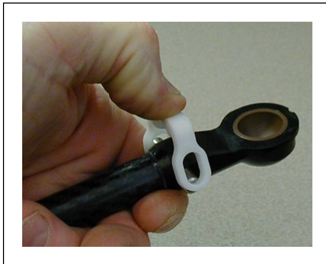
Figure 10-15. Squeezing the Horseshoe into Position, H Shown
