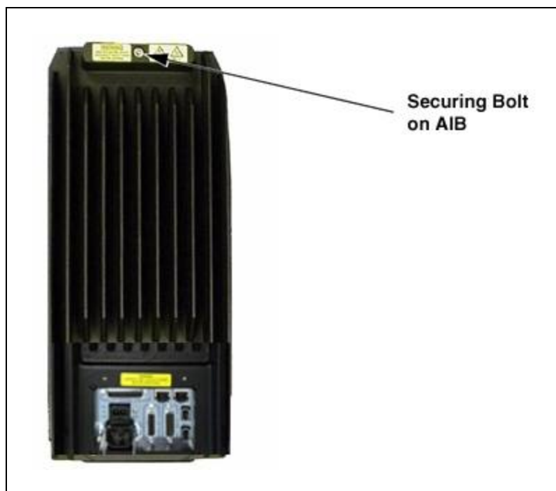
Figure 9-4. Securing Bolt on Chassis
