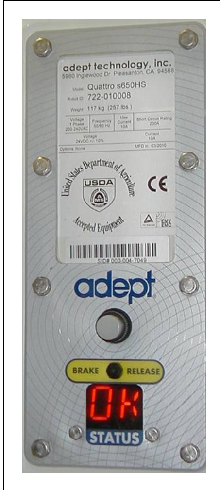
Figure 10-8. Status Display Panel, Showing 8 Hex-head Bolts
