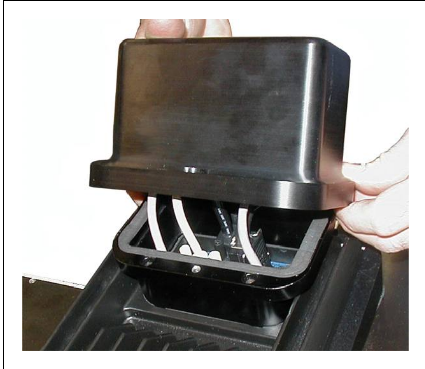
Figure 11-10. Installing Cable Entry Top Cover Assembly
