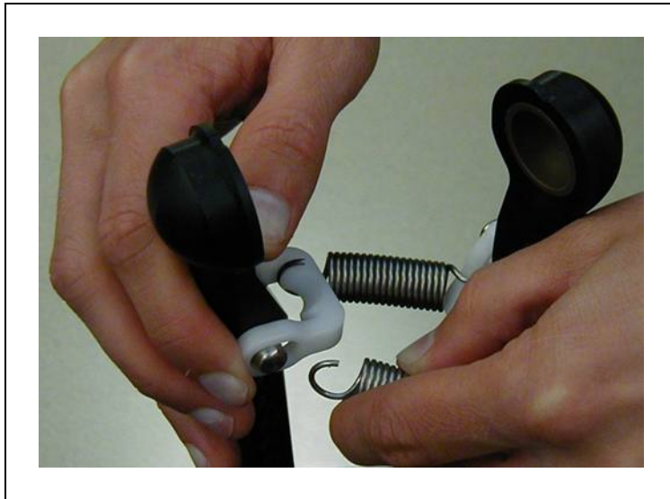
Figure 9-13. Spring, with End Removed from Horseshoe
