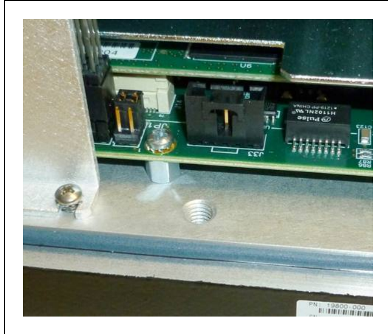
Figure 10-5. Ground Screw Hole on eAIB Chassis
