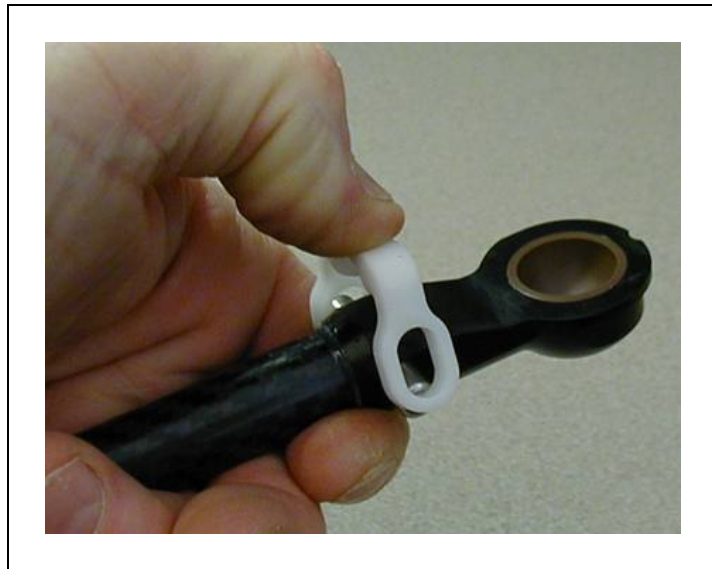
Figure 9-16. Squeezing the Horseshoe into Position
