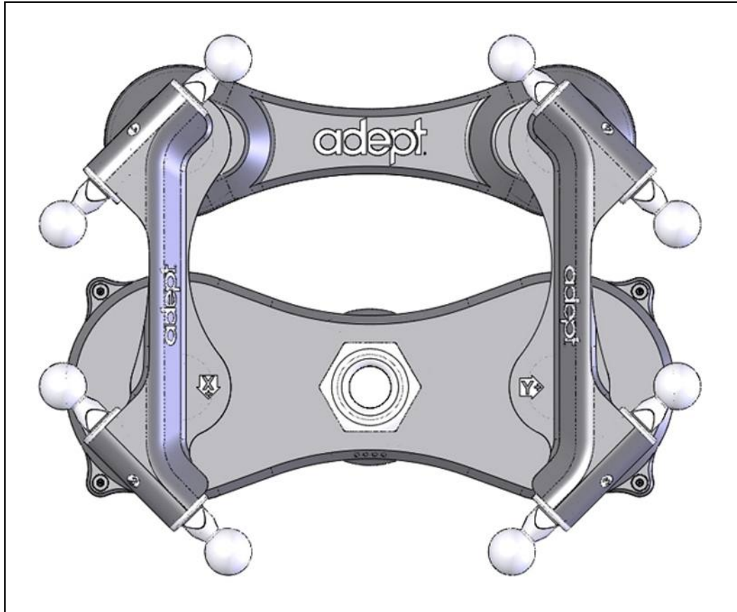
Figure 3-6. Platform Orientation Labeling (P34 shown)
