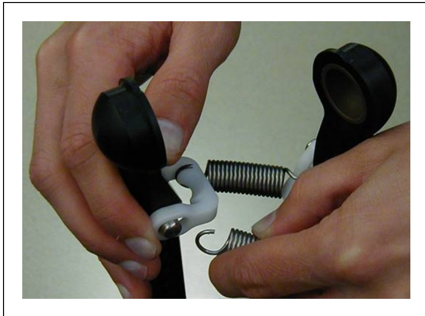
Figure 10-12. Spring, with End Removed from Horseshoe, H Shown
