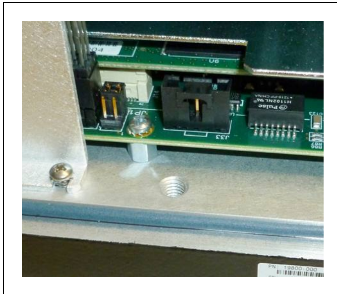
Figure 9-7. Cable Ground Screw Hole on eAIB Chassis
