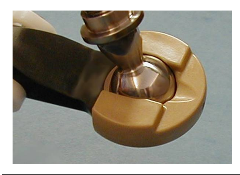
Figure 7-2. Ball Stud Lock on Ball Joint Socket
