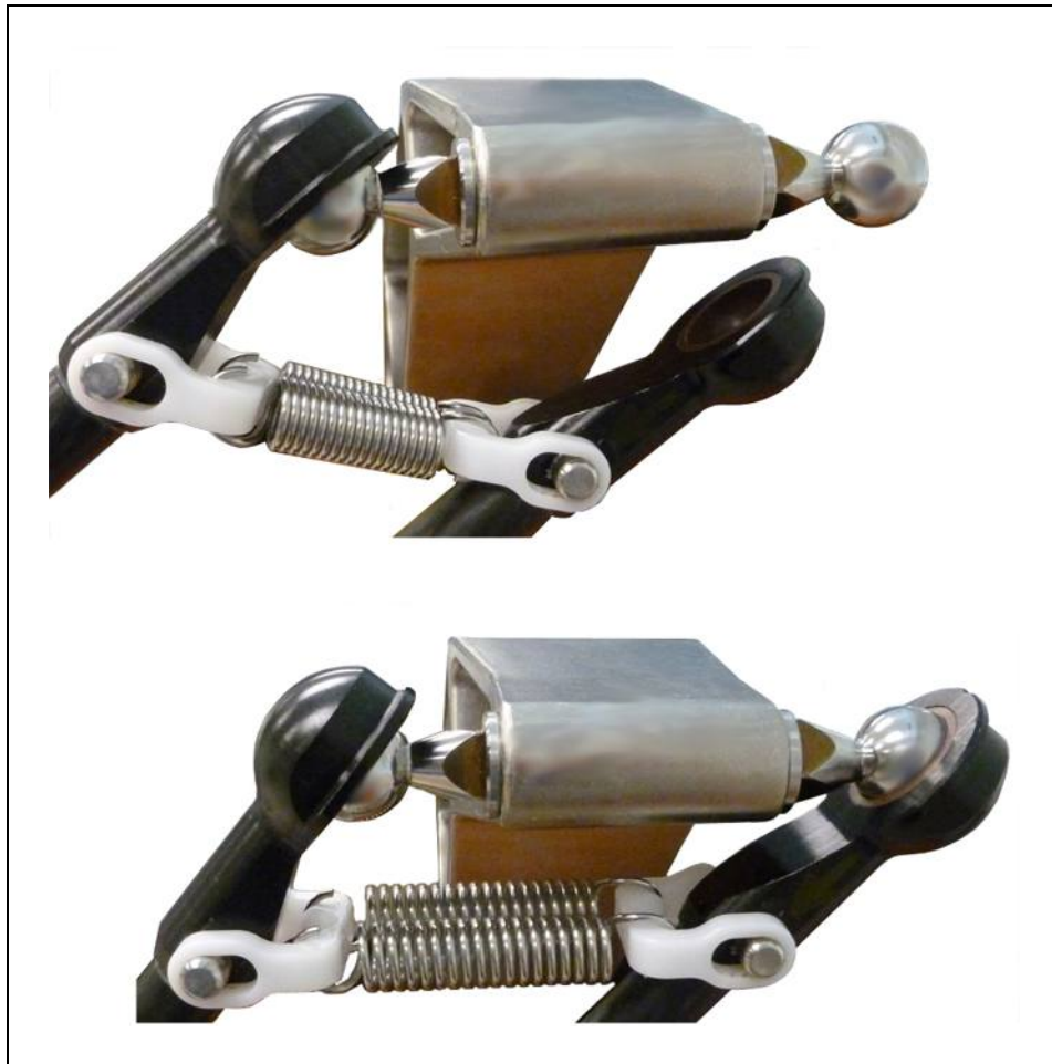
Figure 3-8. Installing Ball Joints
