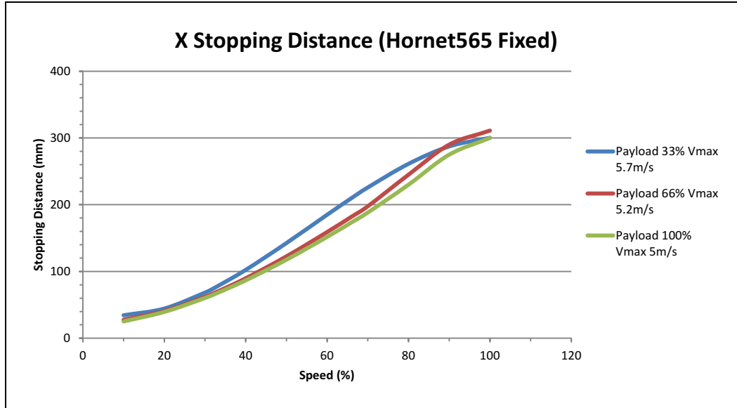
Figure 8-13. Hornet 565 X Stopping Distance with Fixed Platform
