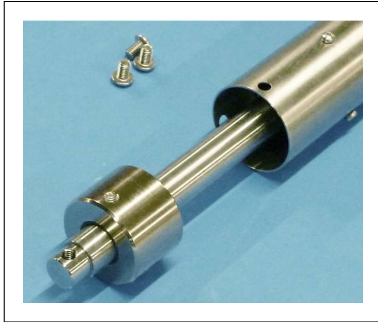
Figure 7-6. End Cap Placed Over Center Shaft
