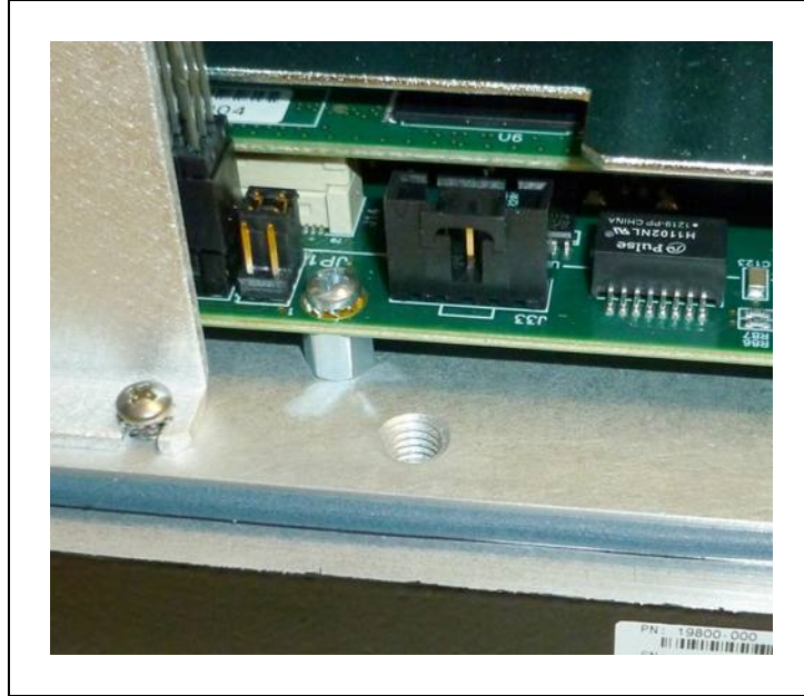
Figure 7-19. Ground Screw Hole on eAIB Chassis
