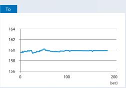
When the automatic filter adjustment function of the E5 D /NX-TC is used, this periodic temperature variation is suppressed automatically. It becomes possible to perform stable temperature control.
