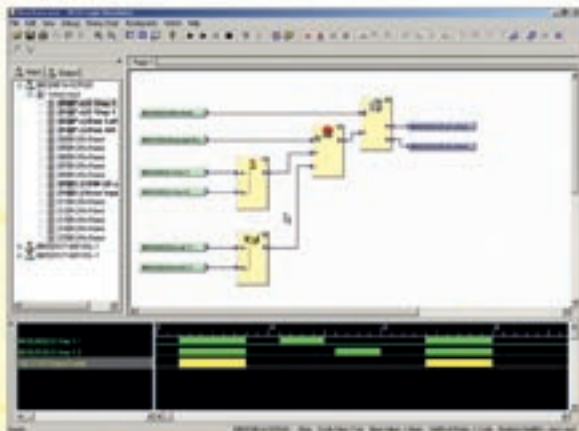
STEP 3 The application program is tested with the logic simulator
