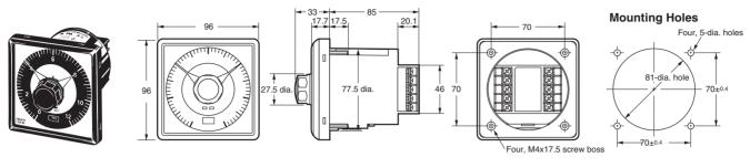
Note: Tightening torque for panel mounting is as follows: 300 m N·m  $\pm$ 50 m N·m
