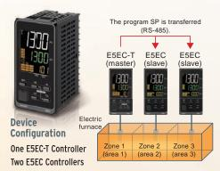
You can easily achieve zone (area) control with component communications. RUN/RESET status of master TC and slave TC link to achieve consistent furnace temperatures in order to improve productivity and reduce lead time.
