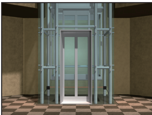
Elevator cage detection
